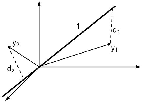
If we now move the deviations vectors to the origin, the cosine(s) of the angle(s) between these vectors are the correlations between the variables.
